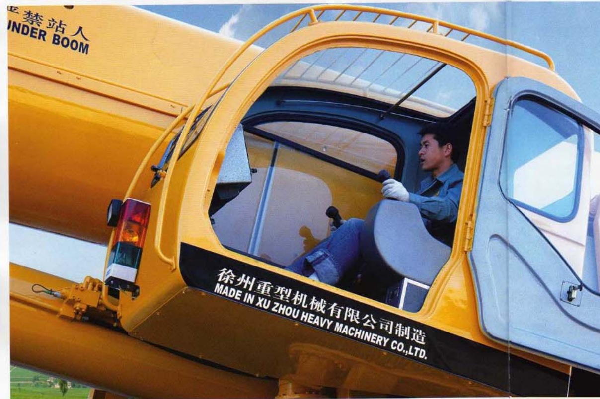
采用第三代改良型操纵室-驾驶室,空间利用更加合理,流线型的外观造型风格统一,与徐工重型独有的圆弧形吊臂相呼应。(可选配三色灯) The third generation of improved type operator's cab and driver's cab, interior space is more reasonable, streamlined appearance and unified style, and with our exclusive oviform boom profile. (three-color lamp is for option)
