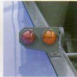
External load lamps Red : 100% of moment Orange : 90% of moment
