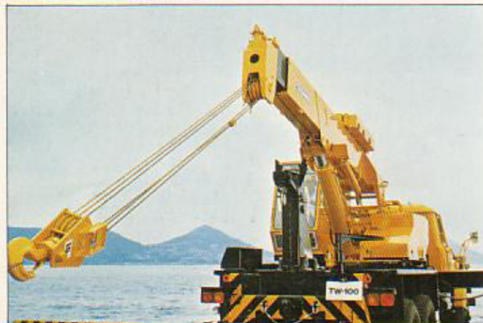
Dragging with the boom and crane winch
