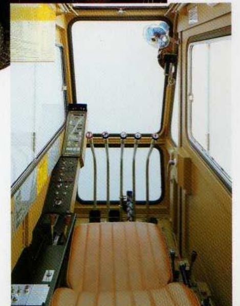
The TG-700E's crane cab. Instrument and control layouts are slightly different from those of the TG-500E.
