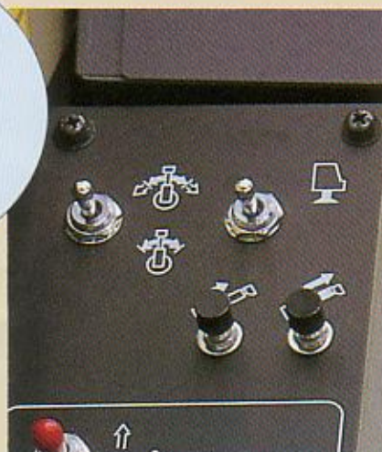
A special switch on the control lever makes it possible to control twin swing easily.
