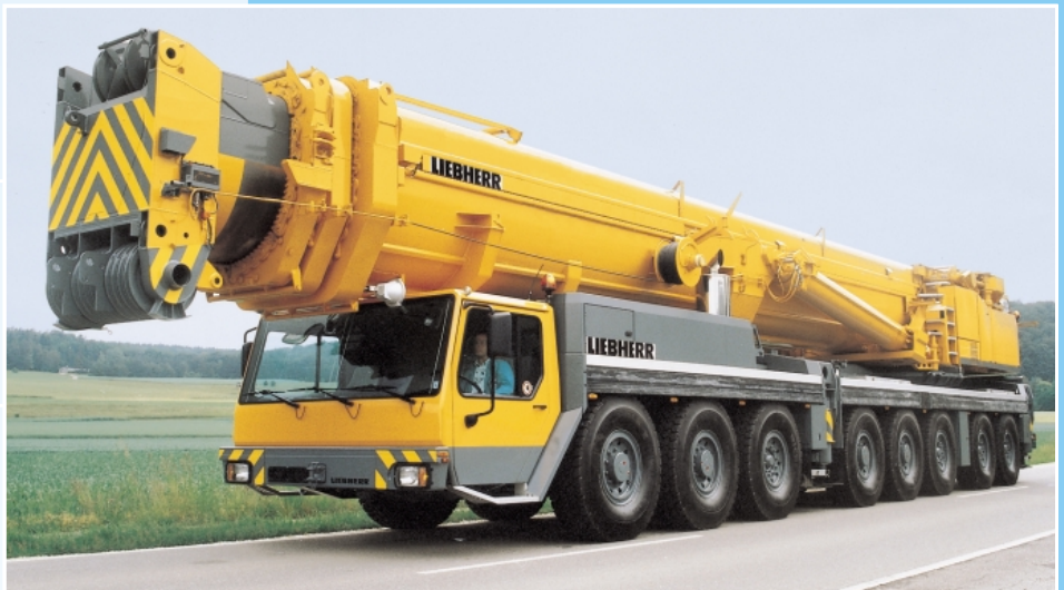
Mobile crane type LTM 1500
