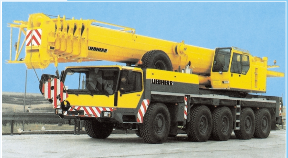
Mobile crane type LTM 1120/1
