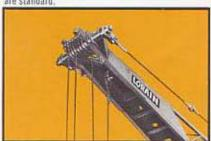
Long-tapered boom tip is available for maximum reach and capacities. Five boom head sheaves are standard Additional sheave available.
