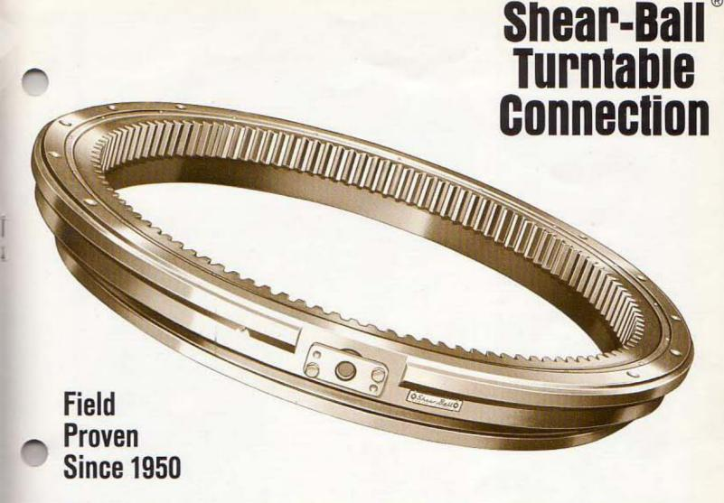
The "Shear-Ball" connection is of exclusive Lorain design. Like a huge ball bearing it allows the turntable to revolve smoothly and accurately. One race is attached to the carrier... the other to the turntable... with balls interlocking the two races and anchoring the turntable to the mounting. All load-forces are dis-
