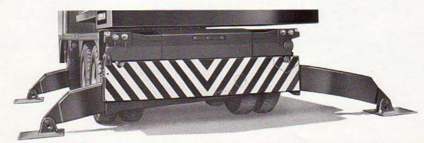
The new Verti-Power Set Outriggers, that are available as an alternate, retain all of the proven advantages of the time-tested Power-Set Outriggers plus added vertical motion for even greater on-the-job versatility.
