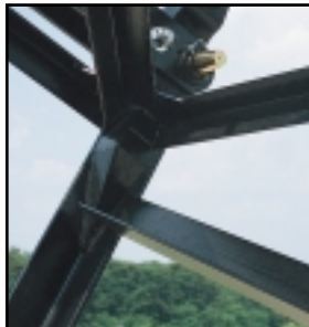
Seamless welds and treated hardware throughout attachment
