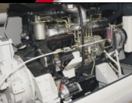
207 hp Isuzu A-6SD1T-QB engine
