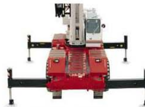
Fully Extended Outriggers 22' 0" (6.71 m) Spread
