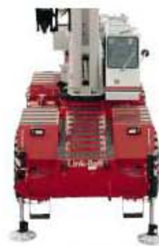
Fully Retracted Outriggers 9' 3/4" (2.76 m) Spread
