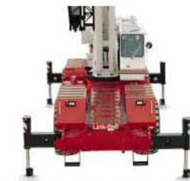
Intermediate Extended Outriggers 15' 6" (4.72 m) Spread
