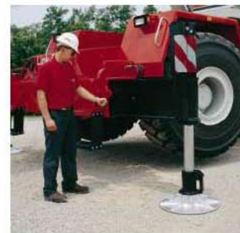
Fully Extended Outriggers 22' 0" (6.71 m) Spread
