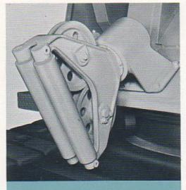
Full-revolving fairleader—rotates to assure full cable support in all positions. All moving parts mounted on anti-friction bearings. Saves cable, promotes greater economy in dragline operations.
