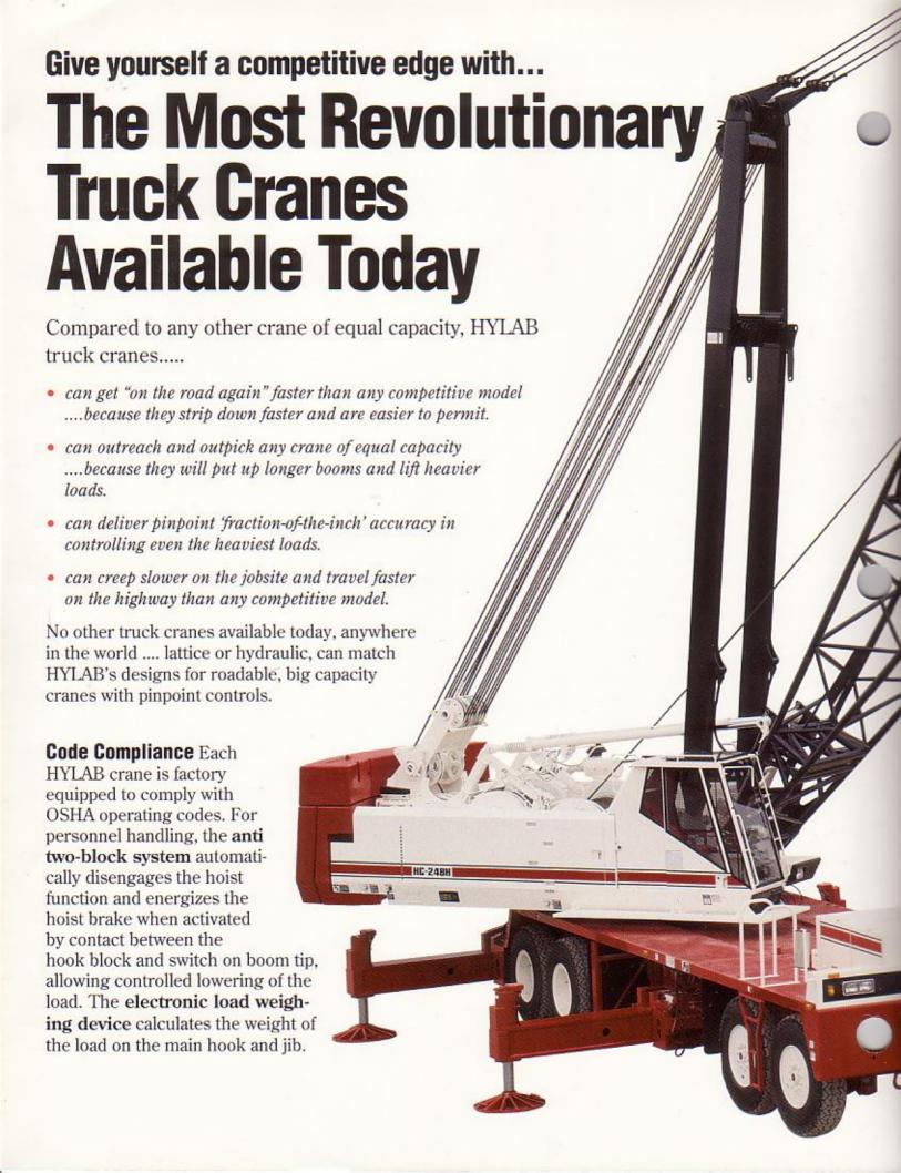
Carrier A revolutionary, deep channel, triple box carrier design provides the optimum strength essential to maximize lift capacity while yielding lightweight axle loadings necessary to meet the most strict highway regulations.
