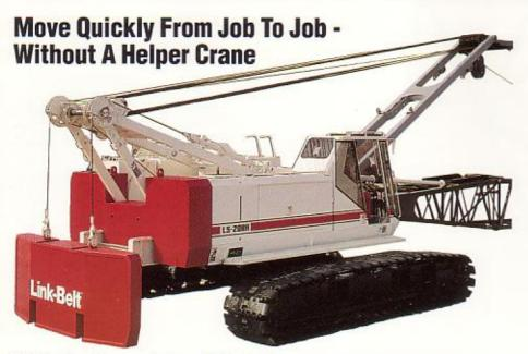
Minimize Dimension and Weight To reduce overall weight for transport, the counterweight can easily be removed with the selfcontained counterweight removal system.
