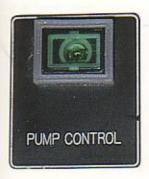
Fine Inching Control For super precise control of load lowering/hoisting, boomhoist or travel, hydraulic pump flow can be minimized by activating the pump control switch. This allows the operator to place loads with either the main or auxiliary drums with extreme accuracy.
