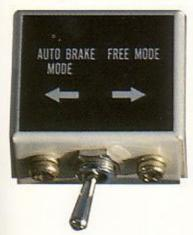
Freefall Mode Select Either automatic brake mode or true gravity controlled freefall mode of operation for load lowering can easily be selected with a conveniently placed toggle switch on the control lever. Freefall mode permits operator to pour concrete on a production basis or drop a hook quickly back to ground level for maximum productivity.
