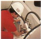
Accessible Collector Ring Quick removal of a protective cover exposes the collector ring, with the boom at any angle.
