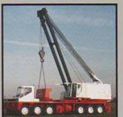
components are removed from the upper and the carrier including: these compoverds rande handled by the live mast, eliminating the need for an additional crane.
