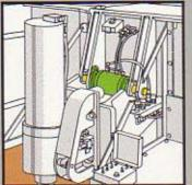
This system employs four double-acting cylinders which are permanently mounted to the carrier frame lugs. Fast, efficient removal or installation of outrioger boxes is insured.
