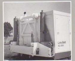
sylinders are stored vertically at the rear of the upper. The entire mechanism remains in place while the crane is on the job or being transported.
