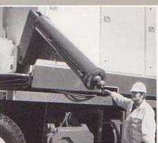
for the entire undecking system is provided by the crane enginepump package. Control is provided (4H 1179.05.1221) ently located valves.
