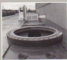
Link-Belt's patented quick disconnect turntable bearing permits connection and release of the upper in seconds - not hours.
