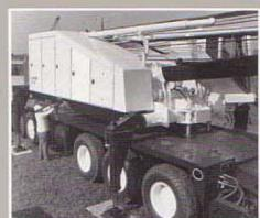
Controls for the hydraulic lift-off mechanism are conveniently located on the right side of the upper.
