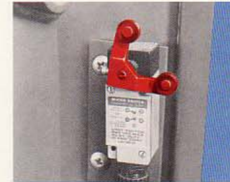
Boom hoist limiting device
