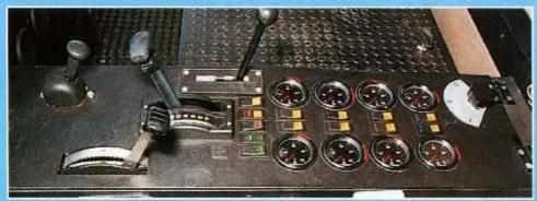
The LTM 1800 has "Niveaumatik" suspension, a Liebherr development, with remote control. This ensures uniform axle-load distribution, equal-isation of axle loads between pairs of axles, auto-matic levelling of all axles at the touch of a switch, crane superstructure lowering by 150 mm to provide increased headroom, crane super-
