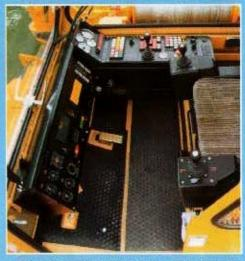
When the crane is operated, the cabin is swung out on a cantilever arm and tilted back to improve the operator's view. Spacious, noise-insulated and equipped with standardised con-trols and instrumentation, this cab satisfies every comfort and safety requirement.
