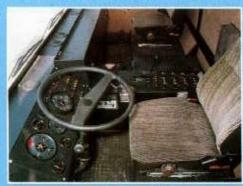
The spacious driver's cab is fully galvanized to prevent corresion, and noise-insulated. The steering wheel is adjustable for height and angle, the controls and instruments are standardized in layout and there are comfortable hydraulically damped seats for the driver and co-driver.
