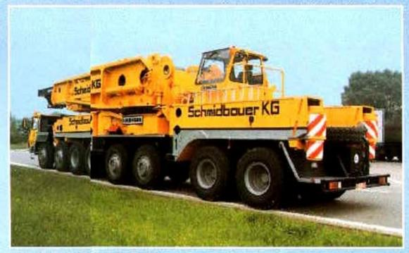
Mobile on the r. with an 8-axle chassis, a 530 hp turbocharged diesel engine, a 5-speed torque-corter transmission and 4 driven and 6 steered axles.
