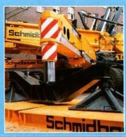
The 4 pivoted arms engage with the base of the frame in a star pattern. By transmitting forces direct to the struts in this way, there is no torsional load on the chassis, and elasticity remains constant throughout the slewing range.
