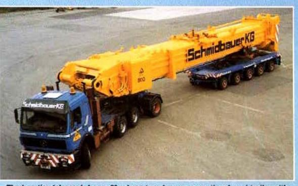
The 4-section telescopic boom, 60 m long, travels on a conventional semi-trailer with steered trailing axie. The supports on the trailing axie turntable and the fifth wheel are of simple pattern, without hydraulic levelling.
