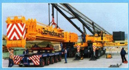
Installing the telescopic boom is a quick, simple matter. With a tensioning ram on the erecting bracket and chain tackle, the boom is lifted off the semi-trailer and swung along the slowing platform centerline. The erecting bracket is repositioned until the base of the boom locates
