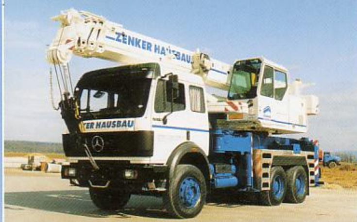
Telescopic crane LTF 1030-3 mounted on a 3-axle Daimler-Benz chassis type 2631 K / 6 x 4.
