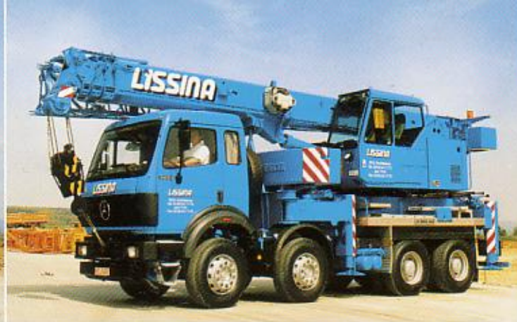
Telescopic crane LTF 1030-4 mounted on a 4-axle Daimler-Benz chassis type 3334 K / 8 x 4.
