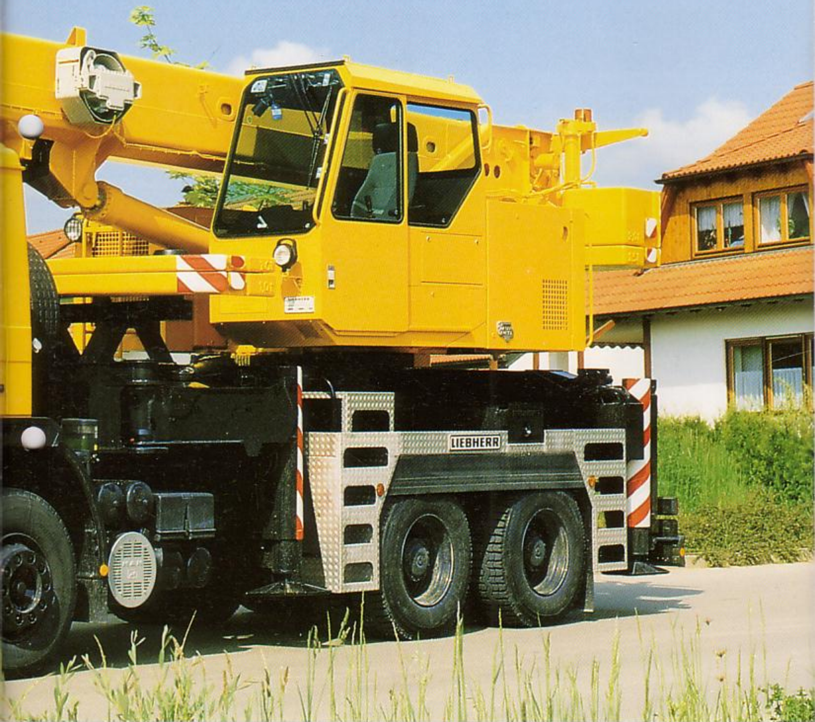
Telescopic crane LTF 1030-3 mounted on a 3-axle Daimler-Benz chassis type 2631 K / 6 x 4.
