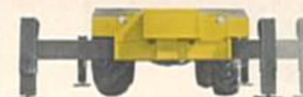
Rugged box-beam type hydraulic outriggers with vertical long-thrust jacks are individually controlled and may be set to match operating situations.
