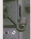
Inching control switch: The lever grips feature an inching control switch for hoist, boom hoist, and travel that the operator can activate without taking his hands off the levers.
